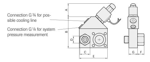
When the hydraulic system is equipped with a closed-centre valve or another type of valve, which has a circulation pressure of 0.15 MPa or more, a separate cooling line must be connected to create oil circulation and cooling of the pump. The connection to the oil tank should be below the oil level.
