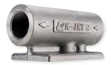
Sunfab Injector K-JET 2 is a basic technical solution for the recirculation of oil in closed hydraulic systems that is cost efficient and saves weight. Three models K-JET 2, cover the flows 160, 250 and 350 I/min.
