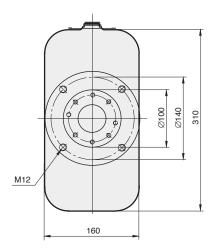
With intermittent operation the gearbox should be filled with 0.5 litres of hypoid oil. Circulation lubrication is required with continuous operation to ensure cooling.
